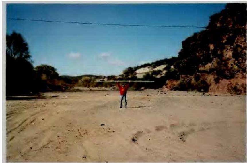
Figure 9E. View upstream from midchannel during no-flow period, Hassayampa River near Morristown. Rod indicates water-surface elevation for the peak flow of January 8, 1993.
